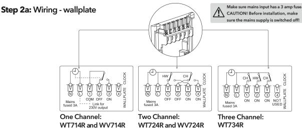
One channel only: Note that the output contacts are voltage-free\*, so power needs to be put on to Terminal 1
