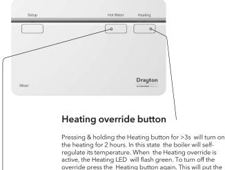
regulate its temperature. When the Heating override is active, the Heating LED will flash green. To turn off the override press the Heating button again. This will put the heating back under system control. Depending on the system settings the heating may stay on which will be indicated by a solid green LED.
