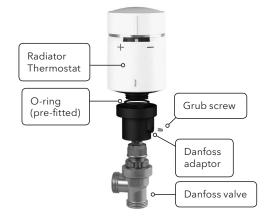
Slide the larger black plastic adapter small end first over the valve. Make sure that the hole containing the grub screw is facing away from you. This way, once its mounted, the markings of the Radiator Thermostat will be in the required position. Use an appropriate size Allen key to tighten the grub screw. Now screw the Radiator Thermostat onto the larger black plastic adapter until tight.
