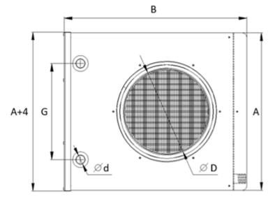
G½" drain is used in water coolers only.
