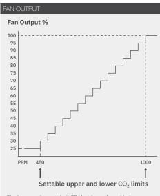
The lower and upper limit CO2 levels can be set between 300ppm and 2000ppm at 50ppm increments. The difference between the lower and upper limit must be at least 300ppm.
